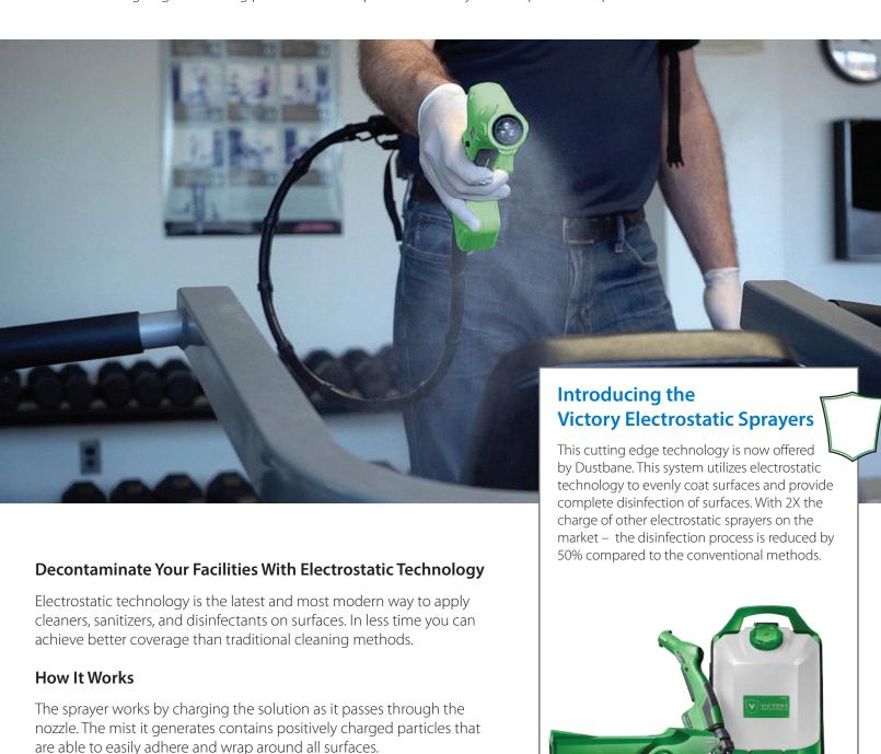
This results in a uniform coating of sanitizer or disinfectant on sprayed objects, including hard-to-reach areas that manual cleaning would miss.
