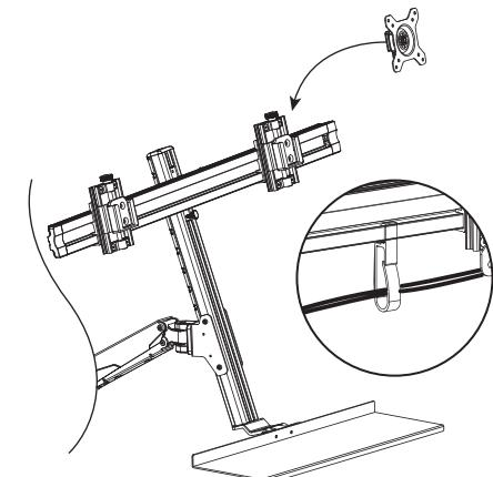
Insert the monitor interface into the slot.
