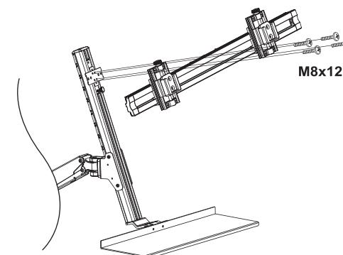
Attach the aluminum horizontal mounting bar to the EFD+2 mounting adapter with the screws provided.
