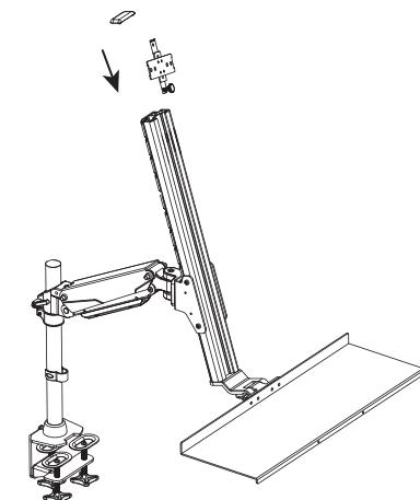
Insert the EFD+2 mounting adapter and replace plastic end cap.
