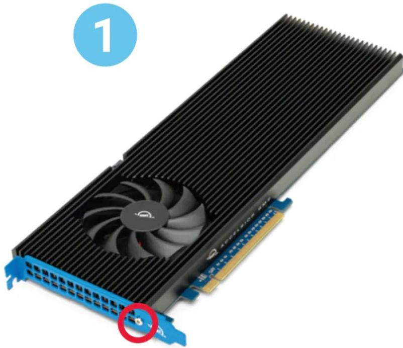
2. Carefully flip the device over and remove the two highlighted T8 screws to loosen the connection with the heat sink.
