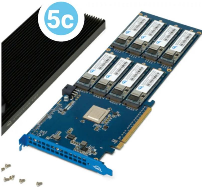
**6.** Set the PCIe card in front of you oriented as shown. Rotate the heat sink so that the drives align with the thermal pads. Next, carefully set the heat sink down on the PCIe card so that the six screw holes on the heat sink are over the corresponding holes on the PCIe card. You may need to press the heat sink down with light pressure to ensure the unit is flush.
