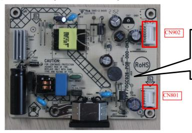
**Warning:** After unplugging the power supply, the capacitance is still charged, do not touch and discharge the capacitor.
