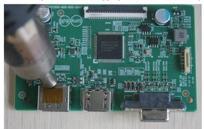
2) Use a hot air gun to melt the solder on the pins.
