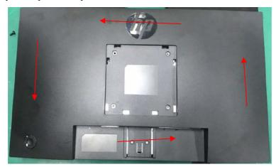
4) Disassemble the Rear Cover and disconnect the connectors.
