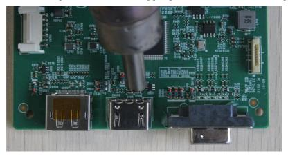
2) Use a hot air gun to melt the solder on the pins.
