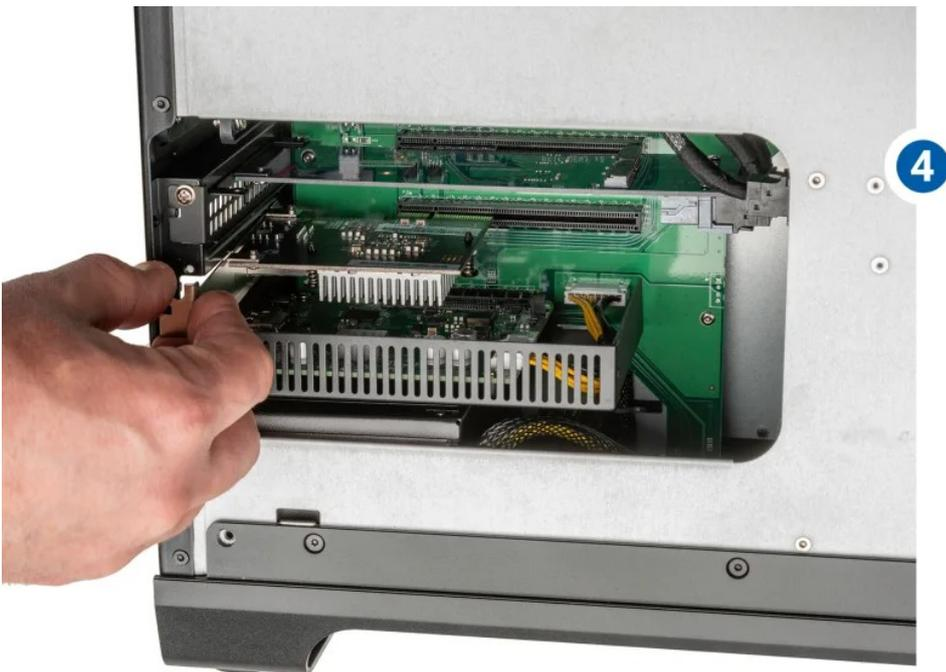
5. Use the screw from Step 3 to affix the card's bracket to the case.
