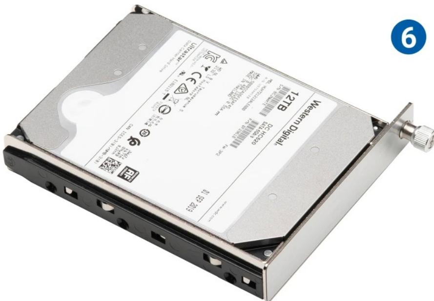
7. Fasten the drive into the drive tray using six of the included screws (three per side). 2.5-inch drives require four of the fine-thread screws.
