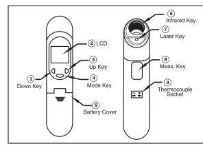
Simply aim the thermometer at the measure target with Lens (6) and press Meas. key (8) to display the surface temperature.
