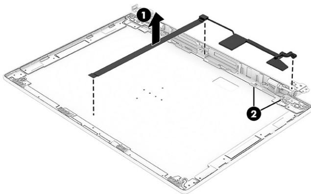
17. To remove the wireless antennas and cables:
