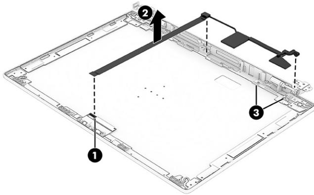
16. To remove the display panel/camera cable on models with an FHD camera:
