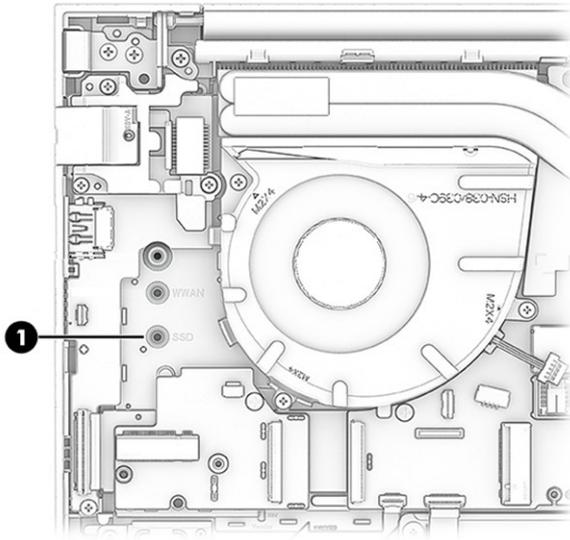
2. Install the screw holder **(1)** in the screw boss for 2230 SSDs.
