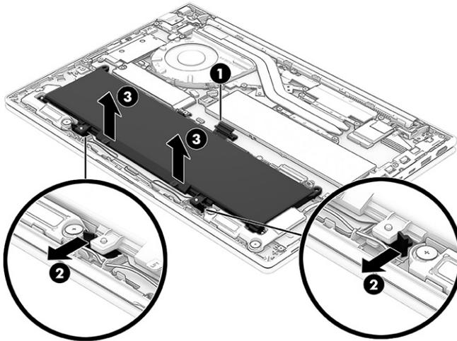
4. To remove the battery latches, rotate the latches (1), and then use a tool to release the latches (2) from the computer. The removal steps apply to both latches.
