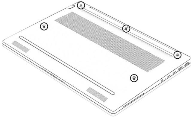
2. Starting near the hinges, use a nonmarking, nonconductive tool (1) to release the edges of the bottom cover from the computer.
