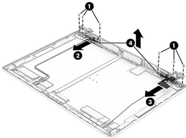
15. To remove the display panel/camera cable on models with an IR camera:
