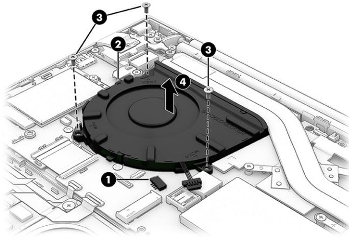
To install the fan, reverse this procedure.
