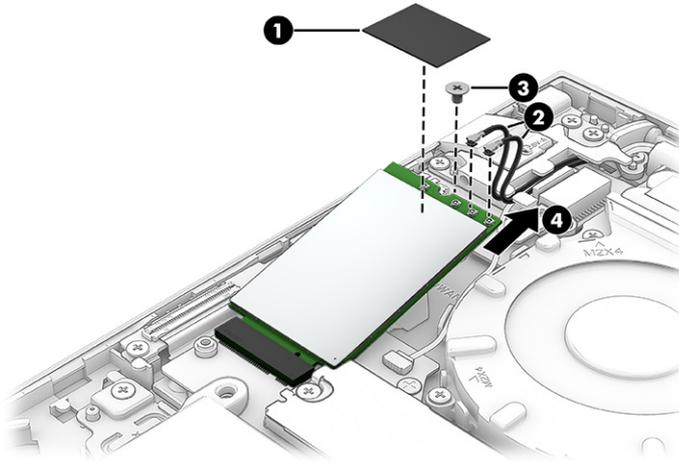
5. If the WWAN antenna is not connected to the terminal on the WWAN module, a protective sleeve must be installed on the antenna connector, as shown in the following illustration.
