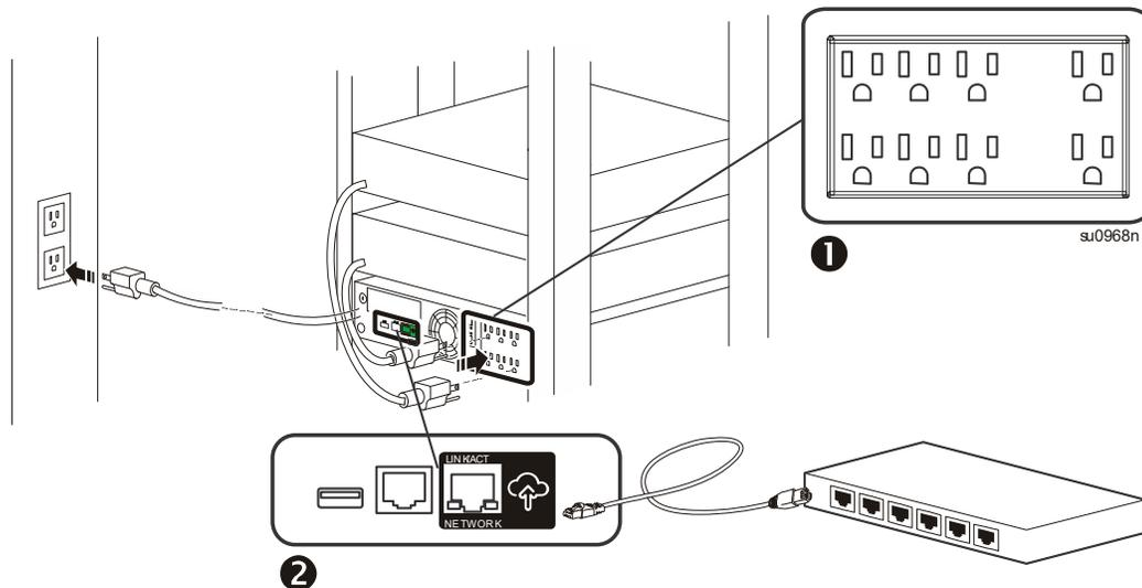
1. Connect equipment to the outlets in the rear of the UPS. Some models are equipped with controlled outlet groups. Refer to the "Configuration" section of this manual for further instructions on the use of controlled outlet groups.
