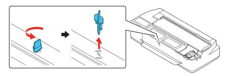
Press the sides of the protective piece, and then lift and remove it.
