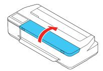
Pull and lift the tab on the ink cartridge cover to open the cover.
