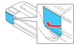
4 Remove the tape and the protective piece.
