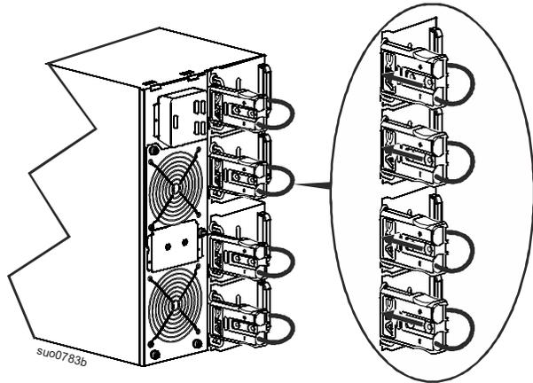
❸ Reinstall the battery compartment doors. Tighten the thumbscrews to secure the doors.
