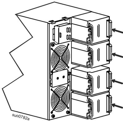
❷ After the UPS is hardwired to branch circuit mains, complete steps 2-5. Connect all four battery modules.
