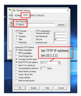
Copy the bundle-axel-SS-8\_10\_130\_0.img file into the TFTP base directory (for example, C:\tftpboot).
