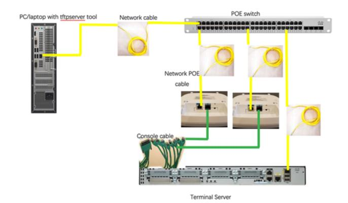
Option 2 - Multiple APs, PoE Switch and USB Hub with Multiple USB-to-RS232 Adapters
