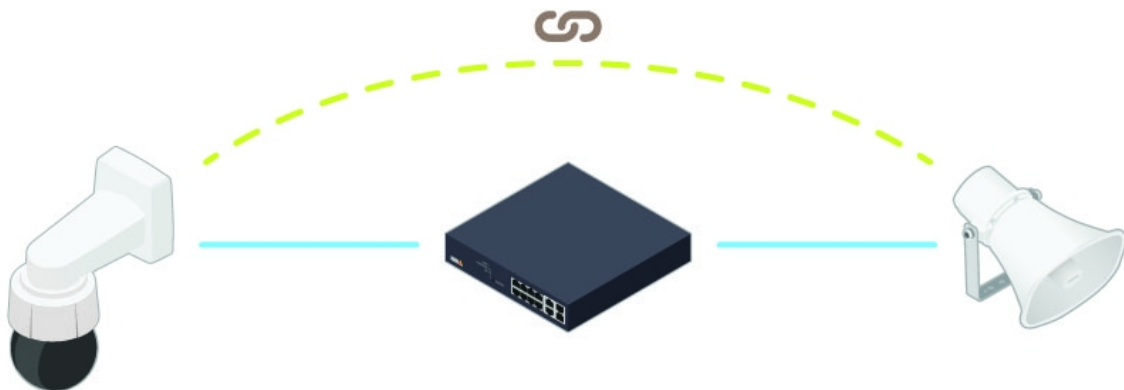
Figure 1. Edge-to-edge technology enables an Axis camera to pair with an Axis speaker to obtain seemingly camera-integrated audio. Both devices must be on the network and the camera must be equipped with edge-to-edge support in the firmware.
