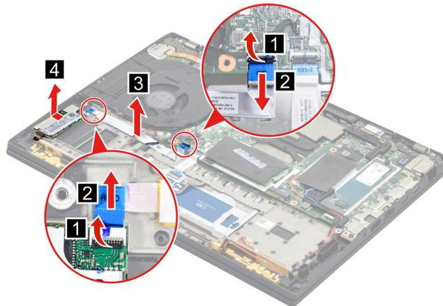
**When installing:** Ensure that the connectors are attached firmly.
