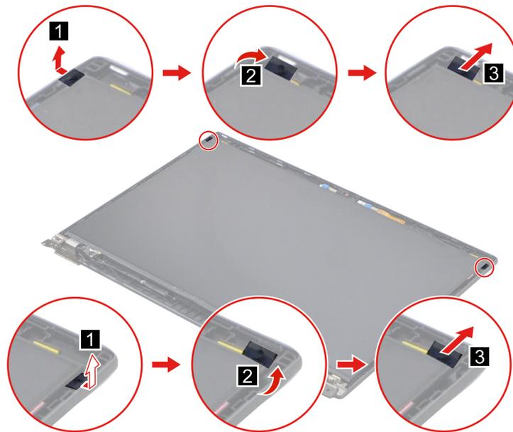
2. Turn over the LCD panel and detach the LCD cable from the LCD panel as shown.
