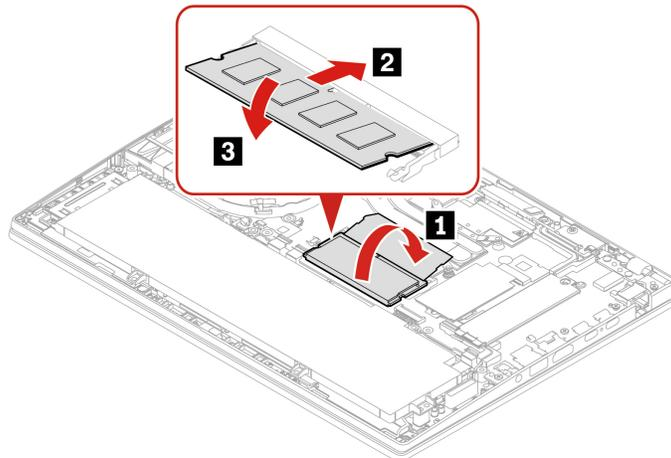
**Note:** Memory module replacement might cause memory retraining during POST. When memory retraining occurs, the screen cannot display the progress information and might be blank. You might see the LED indicators on Esc, F1, and F4 blinking sequentially to indicate the progress. Do not press the power button to interrupt the process. Wait a few minutes until the logo screen is displayed.
