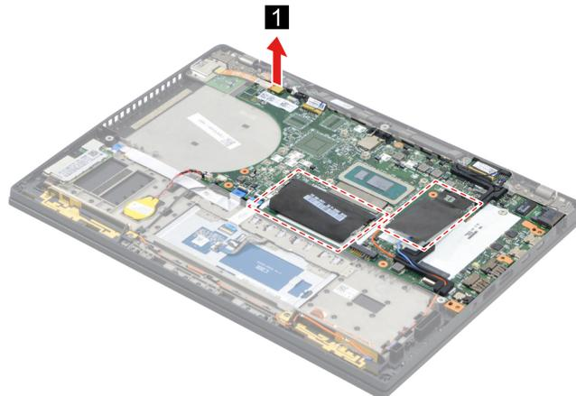
**Note:** Check to make sure all system board mylars and absorbers are taped in place during replacement as shown.
