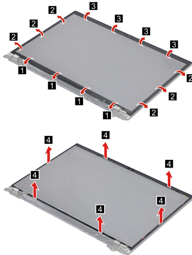
**When installing:** Ensure that all the latches are attached firmly.
