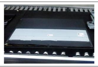
Release the speaker's cable from the hooks, then take out the mylar sheet from Main chassis
