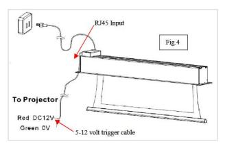
**6.** Wireless 5-12 volt trigger (Item F, Fig 5): The RF remote control serves as a dual purpose, independently as a handheld remote control, or in conjunction with the Wireless 5-12 volt trigger cable. The radio frequency technology can be programmed to send a wireless signal to synchronize its drop/rise with the projector's power cycle.
