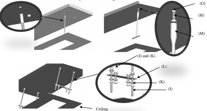
4. Push the screen up into the space. Use the threaded rods (H) to attach the screen assembly to the ceiling. The hexagonal screws (J) will connect the screen to the rest of the assembly. Once firmly in place, use the nuts (I) to ensure a firm connection. Use the socket wrench (M) to make sure that the bolts are firmly tightened.
