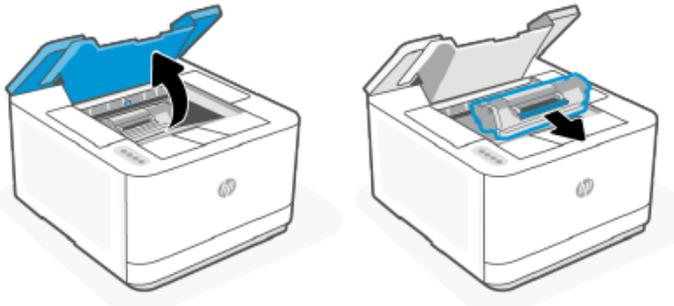
**EN** Power off the **original printer** and remove the power cord from the wall outlet, open access door and remove toner cartridge and install toner in your replacement printer along with all other accessories
