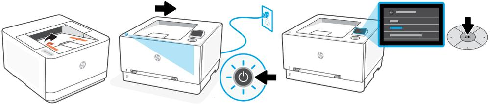
**EN** Remove all tape from the printer. Plug in and power on. On the control panel, choose your language and country/region by using the control pad. Press OK to confirm selection.
