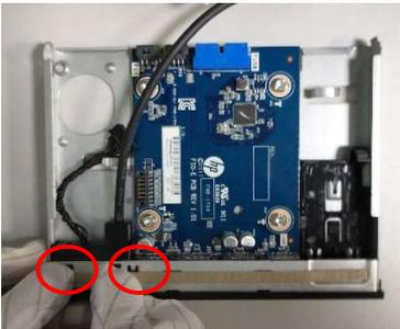
Figure36 Release the front panel mount cable by push out 2 pins fixed black side in switch card tray.
