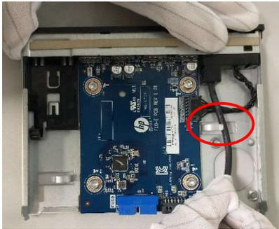
Figure34 Disconnect the front panel mount cable from switch card.
