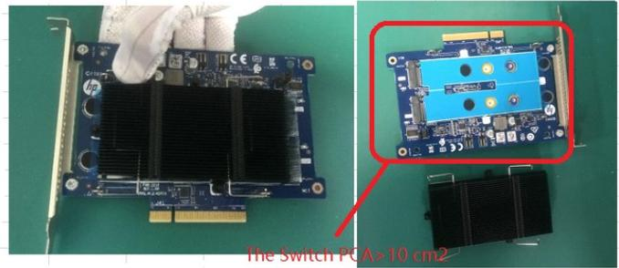
Figure15 Use PH1 screwdriver to uninstall the screws and Z4 G5 Rack DSR.
