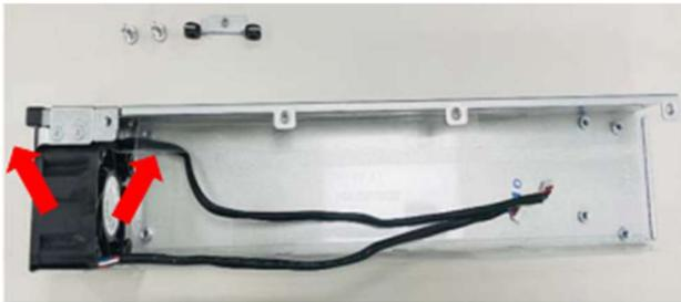
Figure60 Use tool#2 to unscrew two screws to loosen handle-released module from bottom chassis.
