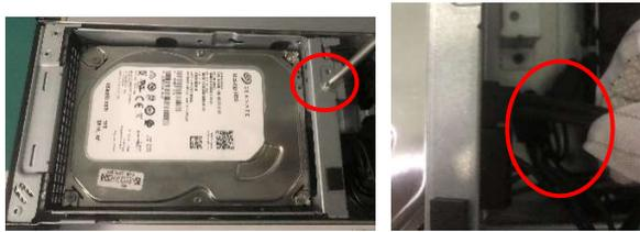
Figure21 Use to PH1 screwdriver to uninstall the screws of HDD.
