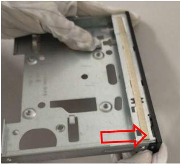
Figure40 Loosen the 2pcs bottom side hooks of switch card panel
