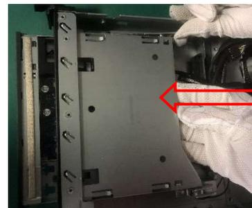
Figure31 Uninstall the screws(x2) of speaker
