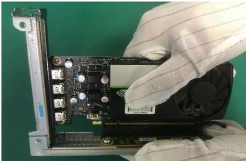
Figure6 Use to PH1 screwdriver to uninstall the screws and detailed parts of graphic card assembly.
