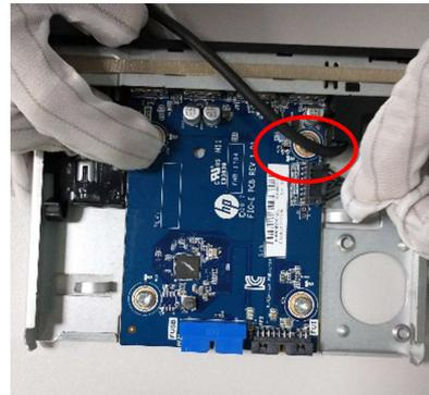
Figure35 Release the front panel mount cable by push out 2 pins fixed front side in switch card tray.
