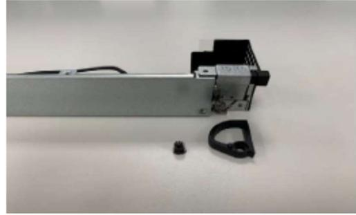
Figure63 Slide handle-released module away from bottom chassis.
