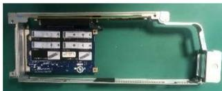
Figure12 Use to PH1 screwdriver to uninstall the screws of extender single slot.
