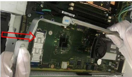
Figure4 Use to PH1 screwdriver to uninstall the screws.
