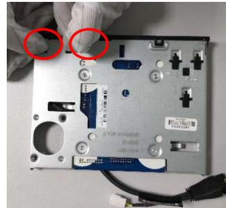
Figure37 Loose the 4pcs switch card PCA screws and remove the switch card PCA
