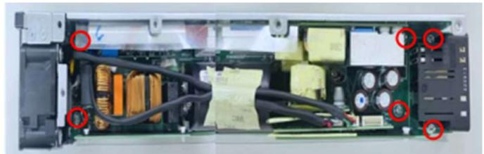
Figure55 Disconnect fan cable connector and LED cable connector from PCBA
