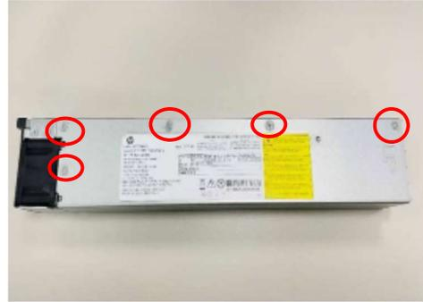
Figure51 Slide top cover to unhook bottom chassis before top cover removal.
