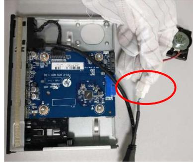
Figure33 Release the front panel mount cable from clip
