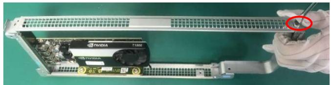
Figure5 Press the graphic card's latch and remove it.
