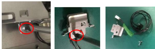
Figure43 Remove the screw with Bosch Power Tools GBM350.
