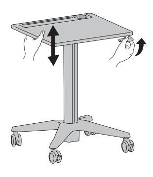
8 Loosen, but do not remove 2 screws to lift and lower hook to desired height.
