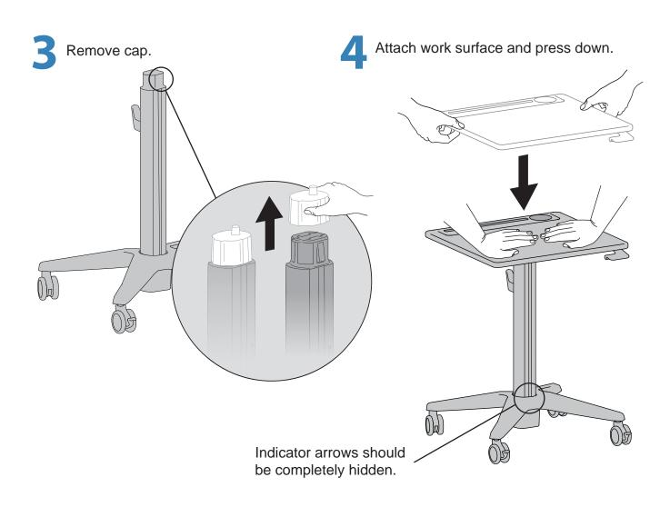
Lift up on the work surface to make sure it is securely attached to the base.
