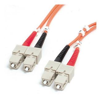
The FIBSCSC2 2-meter (6.6ft) Multimode 62.5/125 Duplex Fiber Patch Cable is terminated at both ends with SC (male) connectors, to provide the necessary connection between fiber networking devices for high-speed, long distance networks.
