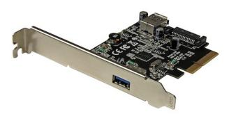
This USB 3.2 Gen 2 card prepares you for the next generation of USB performance, on the inside and outside of your computer. The 2-port card adds one internal Type-A connector as well as one external Type-A connector to your desktop computer, with a combined bandwidth of up to 10Gbps. For power-hungry devices, the card also has an internal SATA power connector, enabling you to use your computer's power supply to add more power to the ports.
