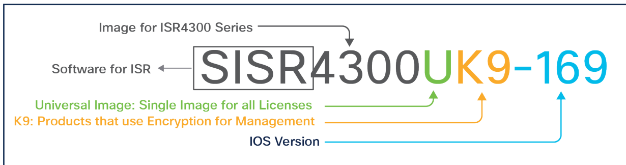
Figure 3. Structure of Cisco Unified Image Nomenclature
