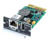
Device monitoring and management, Network Management Cards, NMC3 for Easy UPS On-Line, secure remote UPS monitoring and management
