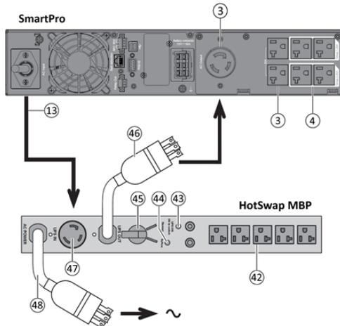
1. Connect the input socket (48) on the HotSwap MBP module to the AC power source.
