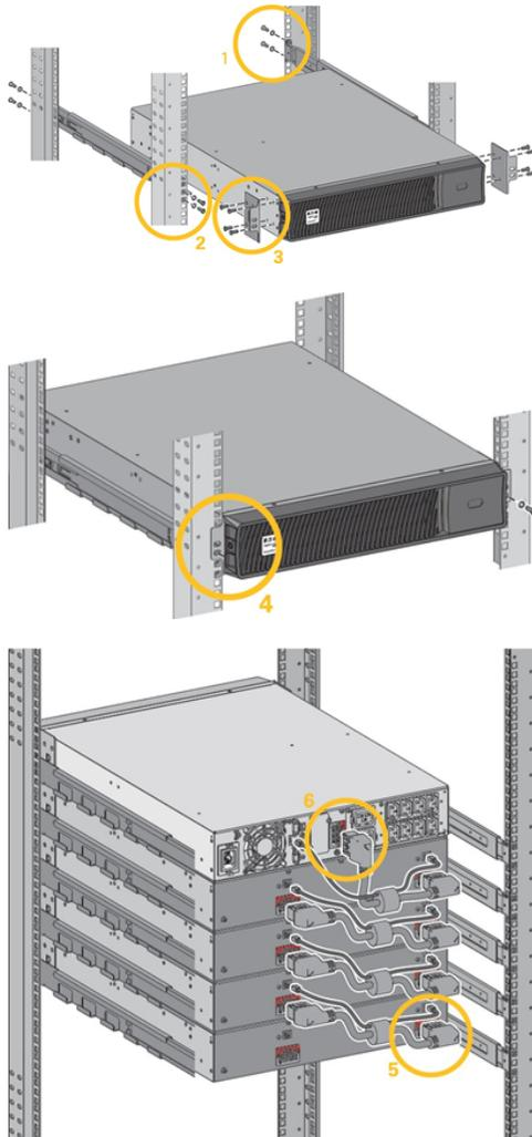
1. Fix the rail on the back of the rack.
