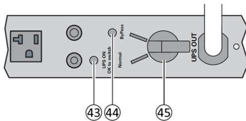
The HotSwap MBP module has a rotary switch (45) with two positions:
