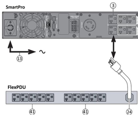
1. Connect the UPS power cord (13) to the AC power source.
