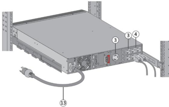
1. Connect the UPS input cable (13) to the AC power source.
