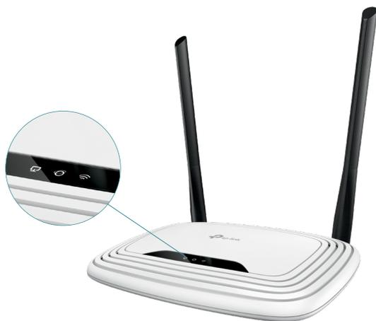
The router's LEDs are located on the front panel. You can check the router's working status by following the LED Explanation table.
