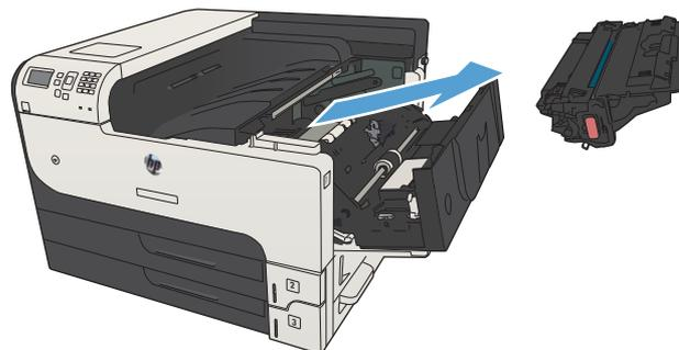
4. Remove the new toner cartridge from the bag. Place the used toner cartridge in the bag for recycling.
