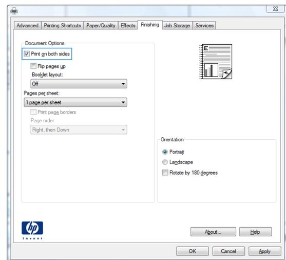
5. In the **Booklet layout** drop-down list, click the **Left binding** or **Right binding** option. The **Pages per sheet** option automatically changes to **2 pages per sheet**.
