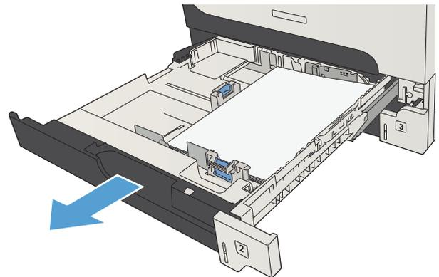
3. Remove any damaged paper from the tray.
