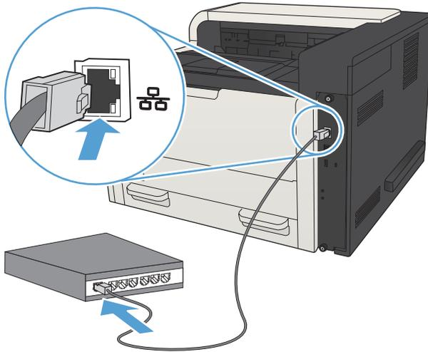
3. Wait for 60 seconds before continuing. During this time, the network recognizes the product and assigns an IP address or host name for the product.
