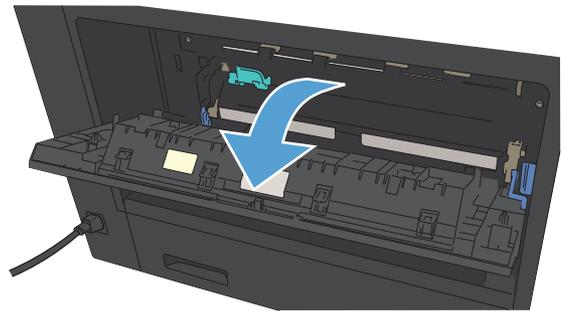
2. Push down on the green tab to open the fuser jam-access cover.
