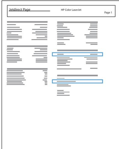
5. **IPv4:** If the IP address is 0.0.0.0, or 192.0.0.192, or 169.254.x.x, you must manually configure the IP address. Otherwise, the network configuration was successful.
