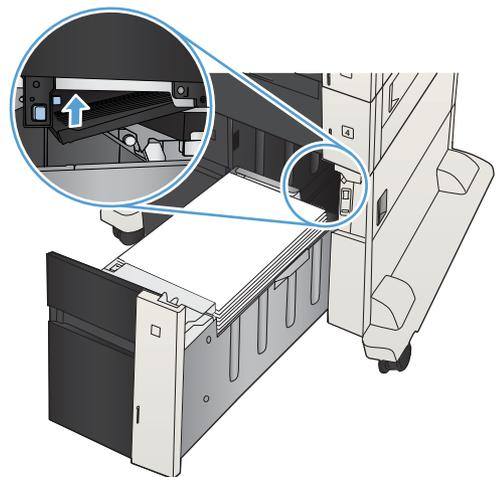
4. If jammed paper is in the feed area, pull it down to remove it.
