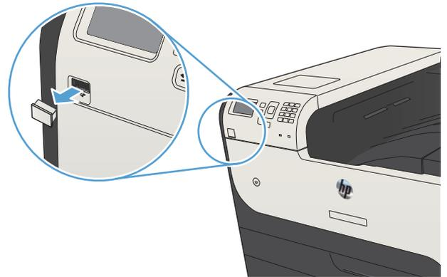
2. The **USB storage device detected** screen opens. Select the **OK** option to access the USB device.
