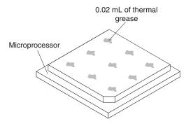
5. Use the thermal-grease syringe to place nine uniformly spaced dots of 0.02 mL each on the top of the microprocessor.
