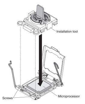
**c**. Twist the handle on the installation tool clockwise and lift the microprocessor out of the socket.
