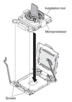
d. Twist the handle on the microprocessor tool counterclockwise to insert the microprocessor into the socket. The microprocessor is keyed to ensure that the microprocessor is installed correctly. The microprocessor rests flush on the socket only if it is properly installed.
