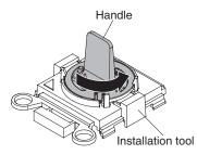
b. Align the installation tool with the screws on the microprocessor socket, and lower the tool on the microprocessor. The installation tool rests flush on the socket only if it is aligned correctly.
