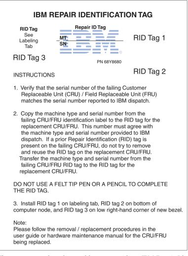
3. The new system-board assembly comes with an IBM Repair Identification (RID) tag. Using a ball point pen, transfer the machine type and serial number from the old system-board assembly to the three labels on the new IBM Repair Identification tag. Place Tag 1 on a label tab (see "Installing a compute node in a chassis" on page 396), Tag 2 on the bottom of the compute node, and Tag 3 on the lower right-hand corner of the new bezel.
