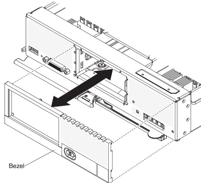
1. Position the bezel on the front of the compute node.
