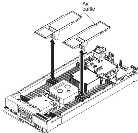
10. Install the air baffle over the DIMM connector.
