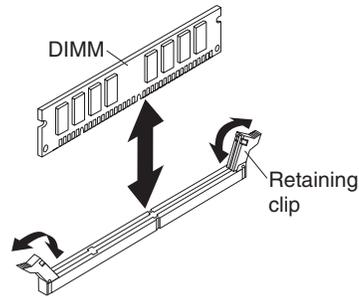
6. Make sure that both retaining clips on the DIMM connector are in the open position.
