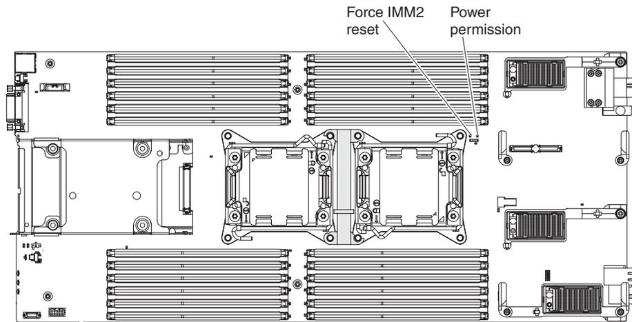
The following table describes the function of each jumper on the system board.
