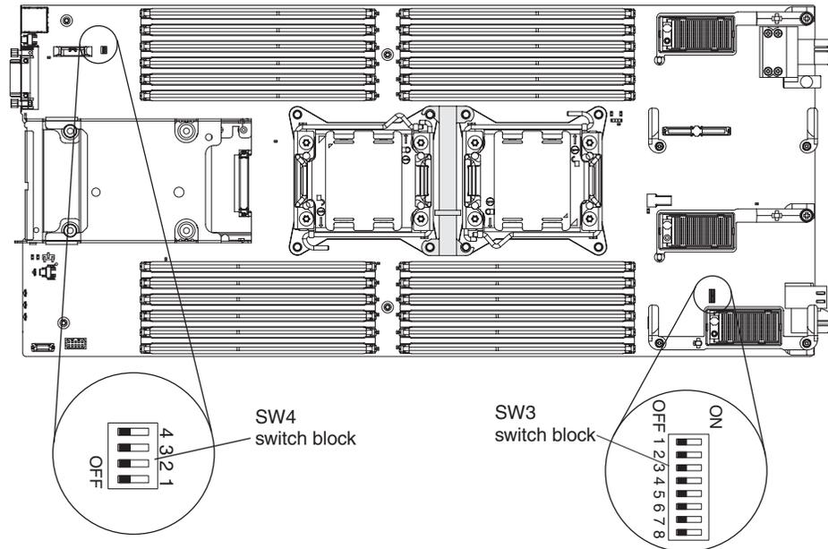
The following table describes the functions of the switches on switch blocks SW3 and SW4.
