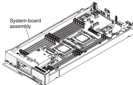
1. Install all of the components in the following list that you removed from the old system-board assembly onto the new system-board assembly.
