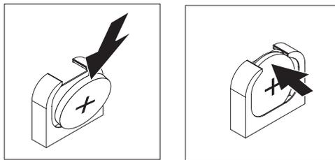
5. Pivot the CMOS battery so that you can insert it into the bottom of the socket.
