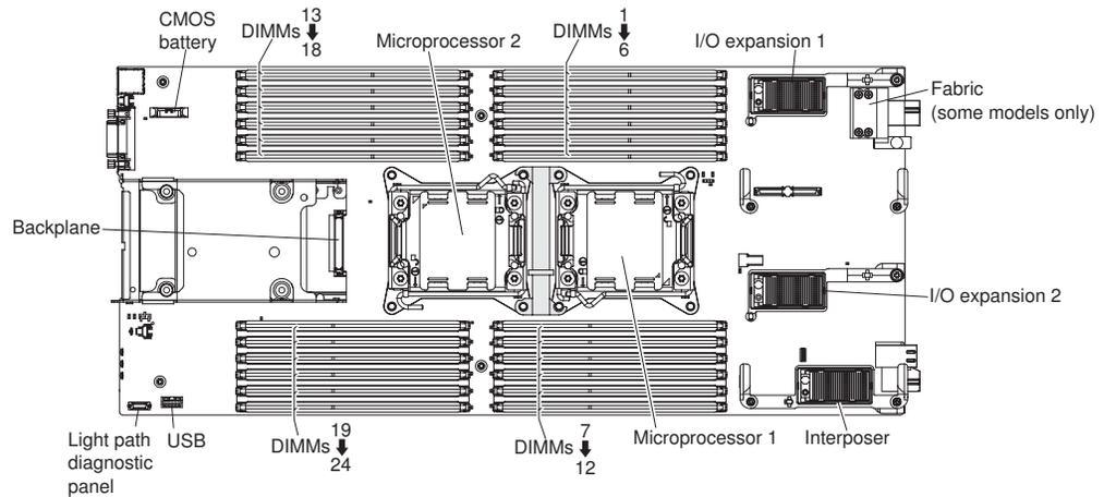
The memory is accessed internally through eight channels (four channels for each microprocessor). Each channel contains three DIMM connectors. Each channel can have a maximum of eight ranks. The following table lists each channel and shows which DIMM connectors are in the channel.
