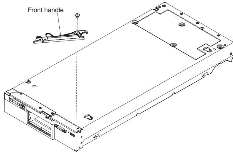
1. Locate the screw that attaches the handle to the compute node.
