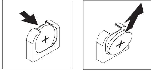
5. Lift the CMOS battery from the socket.
