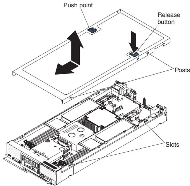
3. Hold the front of the compute node and slide the cover forward to the closed position, until it clicks into place.
