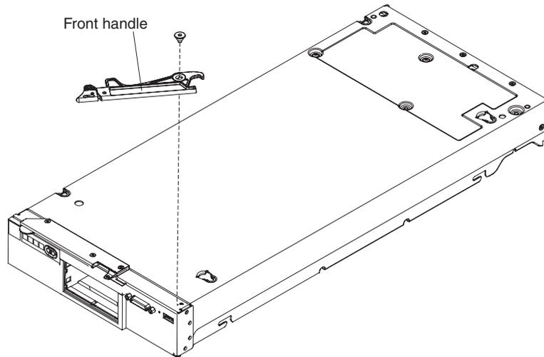
1. Orient the front handle so that the blue release latch is toward the middle of the compute node.
