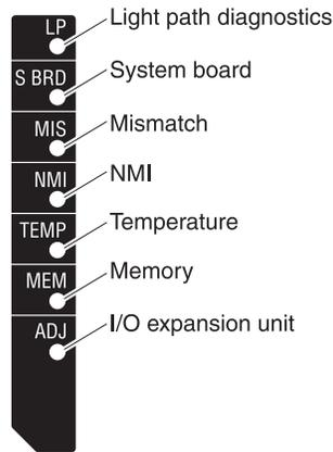
The following illustration shows the locations of the light path diagnostics LEDs on the system board.
