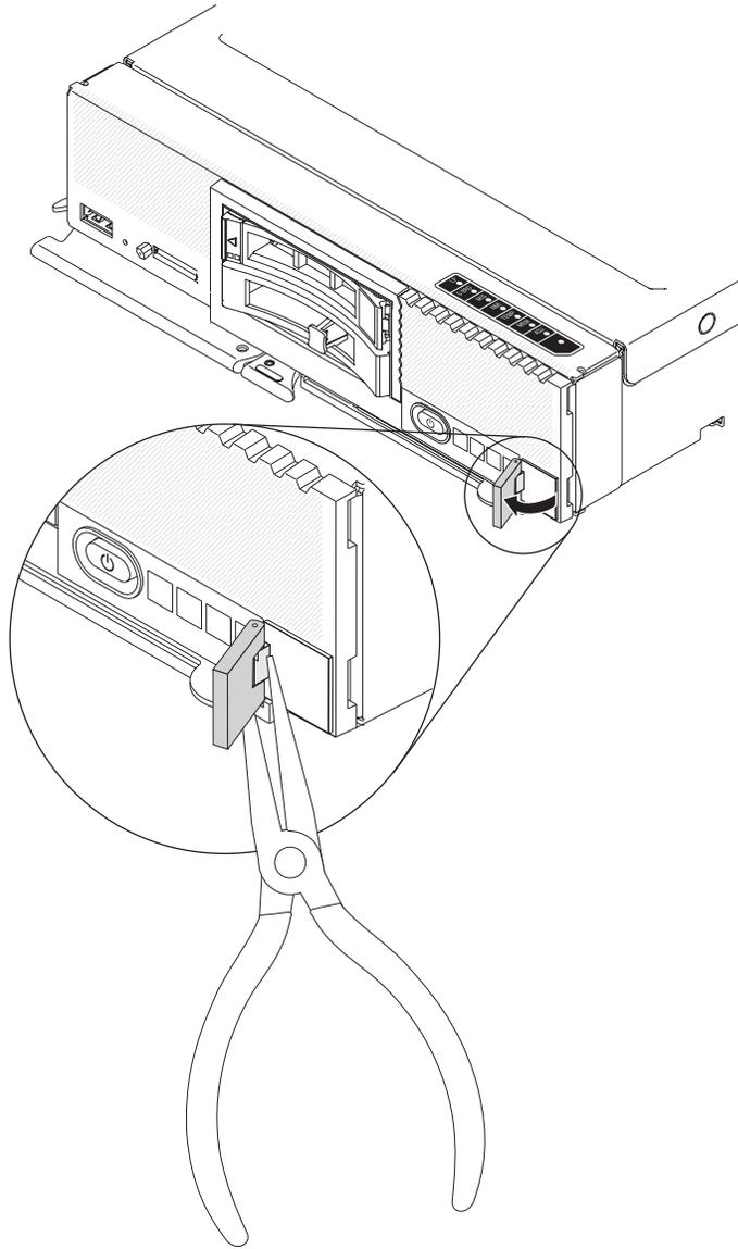
1. If the RFID tag is attached to the hinge, open the RFID tag.
