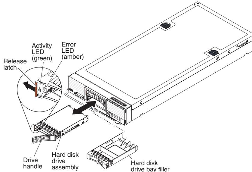
1. Press the release latch (orange) on the hard disk drive to release the drive handle.
