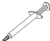
**Note:** 0.01mL is one tick mark on the syringe. If the grease is properly applied, approximately half (0.22 mL) of the grease will remain in the syringe.
