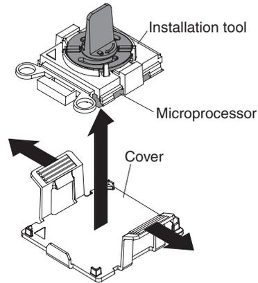
**Note:** Do not touch the microprocessor contacts. Contaminants on the microprocessor contacts, such as oil from your skin, can cause connection failures between the contacts and the socket.
