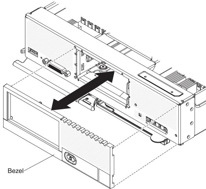
1. Use a flat-blade screwdriver to carefully pull the bezel from the compute node.
