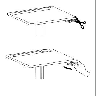
5 Lift brake release lever to raise and lower riser.
