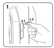
Unlock access panel: to unlock, insert the key provided and rotate counterclockwise ¼ turn.
