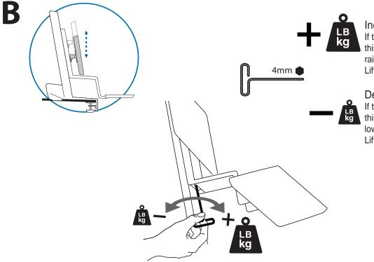
Increase Lift Strength If the mounted weight is too heavy or this product does not stay up when raised, then you'll need to increase Lift Strength:
