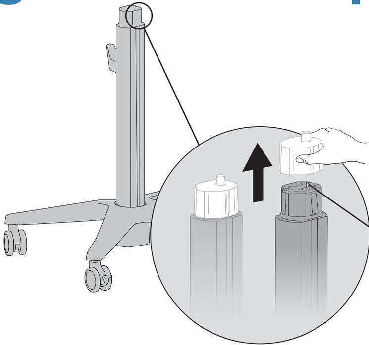
**4** Attach work surface and press down.
