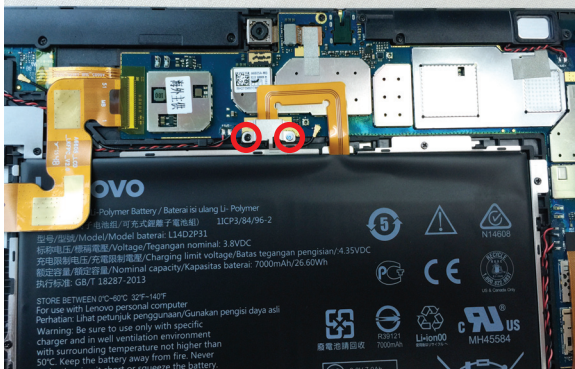
Figure 2. Removal steps of the LCD FPC
