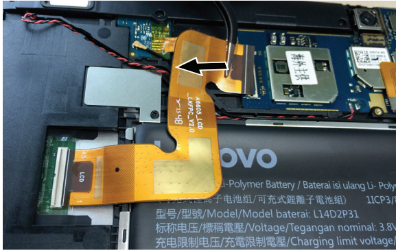
Figure 2. Removal steps of the LCD FPC (continued)
