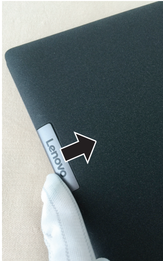
Figure 1. Removal steps of back cover
