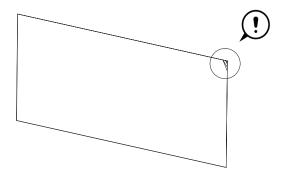
Repeat step 5g). Remove the springs around the corners and move the material towards the corner as shown below. Remount the springs and pull on the fabric manually as described above to get rid of wrinkles in the corner of the fabric. Pull on the fabric and wrap the fabric around the corner until the corner is flat and free of wrinkles.
