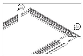
**2d)** After you have joined the two horizontal frames and all four corners, your frame will look similar to below. Check and tighten all Set Screws as you will not be able to access them once the Outer Frame is installed.
