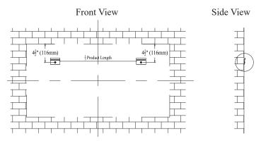
Draw a center line for your screen in the desired location. Mount the Hanging Bracket centered to your screen and 4 1/2" (116 mm) from the top of the screen.
