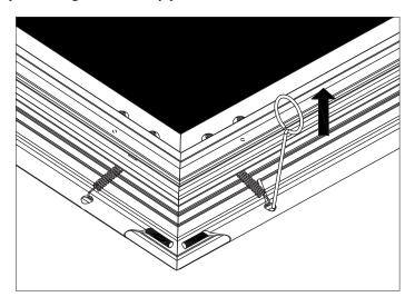
If your screen still has wrinkles or more tension is required, repeat the above method and pull on the fabric harder until you have reached the desired effect.
