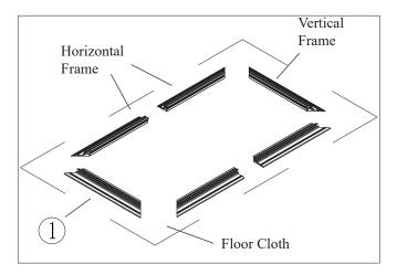
**1b)** Insert two Joint Brackets into the slots of the two horizontal frame pieces. Center the brackets, and then insert the Set Screws. Do not tighten the set screws, as shown below:
