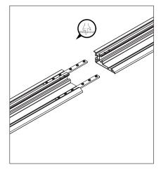
**2b)**Insert the Corner Brackets into both sides of the vertical frame and the horizontal frame. Align the corner pieces and push the two frame pieces together. Make sure there is no gap bigger than 1mm, then tighten the Set Screws.
