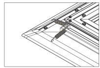
Repeat the above step for all four corners and check if all four corners are free of wrinkles. If the wrinkles still exist, repeat the above steps by pulling on the corner of the fabric a little more.
