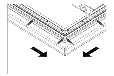
**5i)** At each of the corners of the screen material there will be a flap of material with velcro attached facing upwards. Cut off the excess velcro so that 1/4" of the velcro is left between the frame and the material at the corner as indicated by the arrow below on the left. Flip the flap of material over and stick the velcro towards the frame as shown below on the right.
