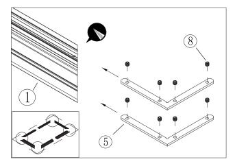
**1d)** Your screen now should look like the diagram shown below. Join the Inner Frame pieces together with the brackets from previous steps.
