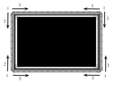
**5d)**Pick a corner to start working at. Mount 4 springs in the 4 holes that are closest to the corner starting with the vertical side (2). Repeat with all 4 corners.
