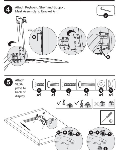
**Note:** Firmly secure the VESA plate to the display using the appropriate screws, washers and spacers (if necessary).
