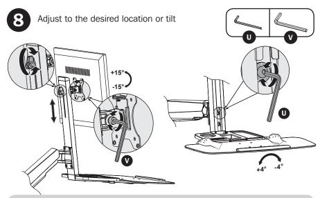
To correct the tilting angle, tighten the adjustment screws using the provided Hex Keys (or tighten the knob).
