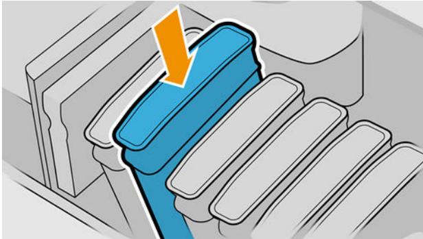
4. Push the cartridge into the slot until it snaps into position.
