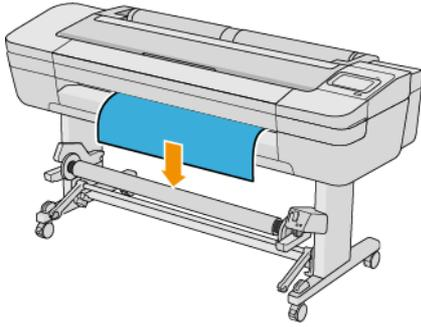
11. Pull down the center of the paper's leading edge to straighten the paper. Do *not* attempt to pull more paper out of the printer.
