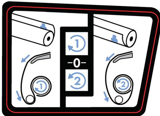
14. Tap the button on the front panel to advance the paper, creating a loop.
