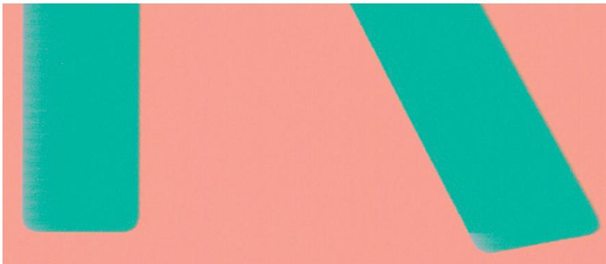
1. If edges of objects or lines appear to be poorly defined or lighter in density, and you have already set the print-quality slider to **Quality** in the driver dialog, select the custom print-quality options, and try setting the quality level to **Normal**. See [Printing on page 59](#).
