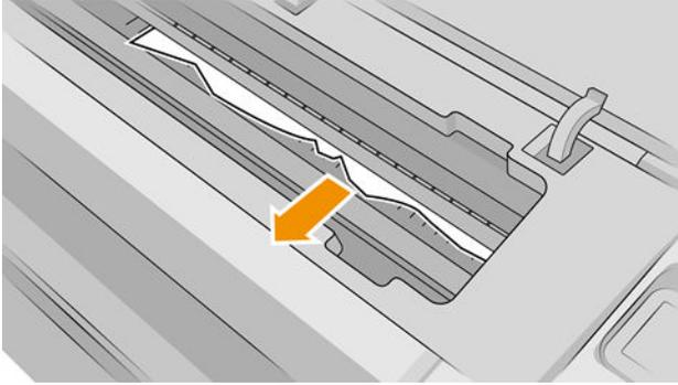
**⚠ CAUTION:** Do not move the paper sideways, as it could damage the printer.
