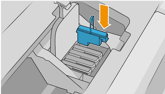
**⚠ CAUTION:** When installing the new printhead there may be some resistance, so you need to press it down firmly but smoothly. You should hear a beep and see confirmation on the front-panel display that the printhead has been inserted. If you have difficulty, see [Cannot insert a printhead on page 170](#).
