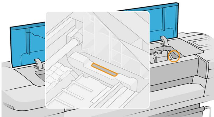
5. Remove any debris blocking the printhead drop detector.
