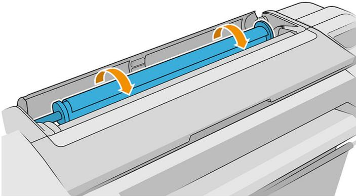
**💡 TIP:** When loading the upper roll, avoid inserting roll paper into the cut-sheet slot. If you do so, the printer beeps and the front panel asks you to remove the paper.
