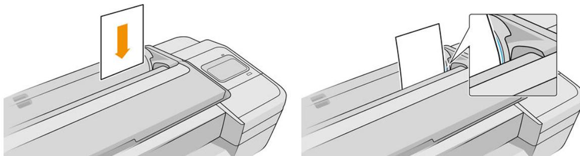
6. Load your sheet aligned with the load line and insert it until the paper will not continue; with thicker sheets, you feel resistance.
