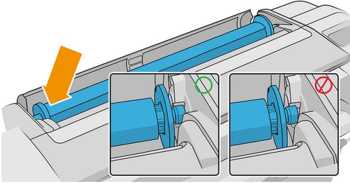
6. With both hands, push the spindle into both roll holders at the same time.
