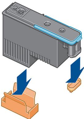
2. The printhead is designed to be inserted into any of the available slots. Once the printhead is inserted into a specific slot, it will be set up to work only with that combination of colors. For this reason, it is important to mark the printhead with its specific color, on the label that comes with it, matching the color of the carriage slot into which the printhead is to be inserted.
