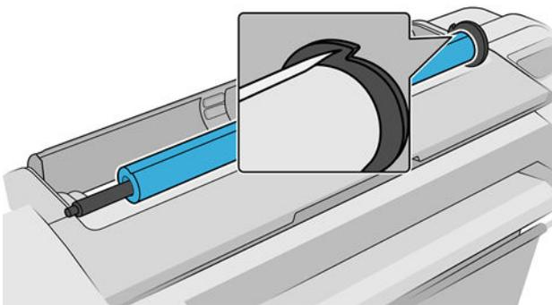
Ensure that the end of the roll is as close to the spindle stop as possible.
