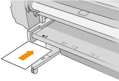
5. Load your sheet aligned with the load line and insert it until the paper will not continue; with thicker sheets, you feel resistance.
