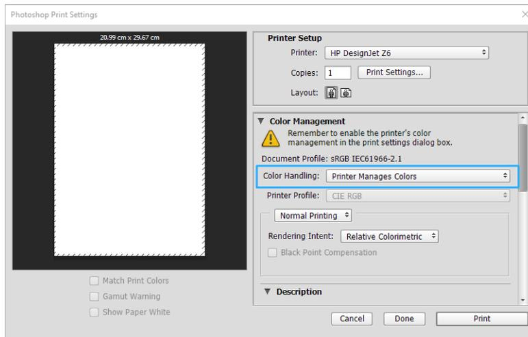
3. In the driver's **Color** tab, ensure that the color management option is **Printer managed colors**. This is the correct option because you have already selected **Printer Manages Colors** in Photoshop.
