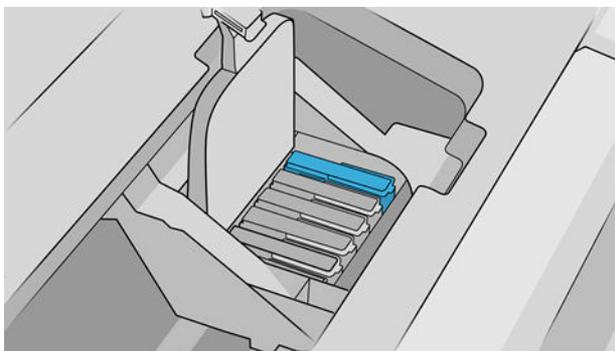
4. Insert all other printheads that need to be installed, and close the carriage lid.
