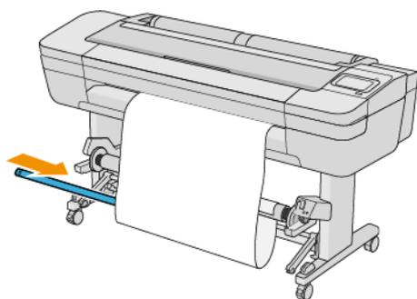
18. Fit the loop shaper into the supports at either side.
