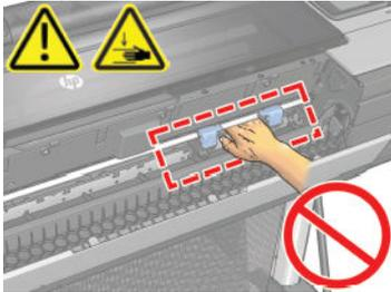
3. To put a module back in place, pinch the latch and insert it into the cutter support.
