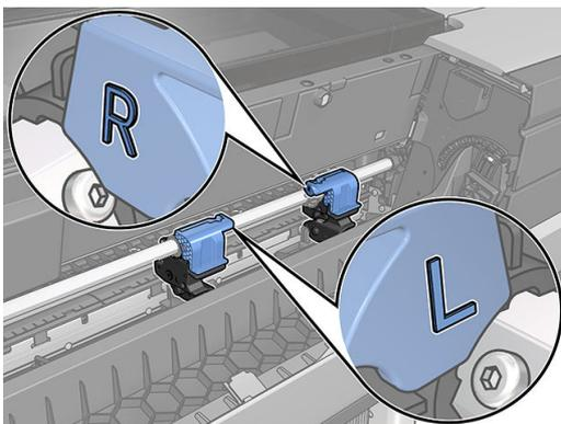
4. Make sure the modules are correctly attached to the bar.
