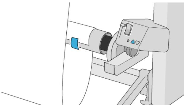
16. Press the button to advance the paper again. The paper should advance until it almost touches the ground.
