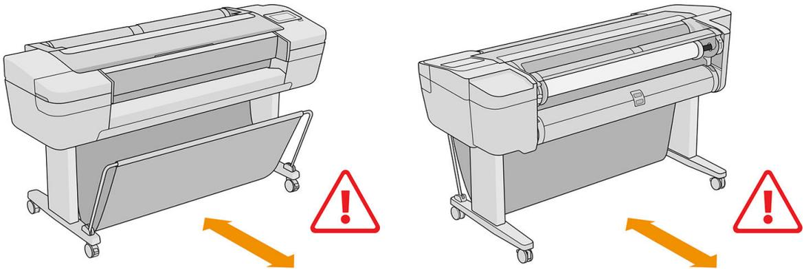
**⚠ CAUTION:** Make sure the printer wheels are locked (the brake lever is pressed down) to prevent the printer from moving.
