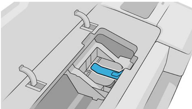
When all the printheads have been inserted correctly and are accepted by the printer, the printer beeps.
