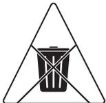
**Do Not Discard:** The UPS or UPS batteries in trash. The batteries contain lead acid. For more information, contact your local recycling or hazardous waste facility.
