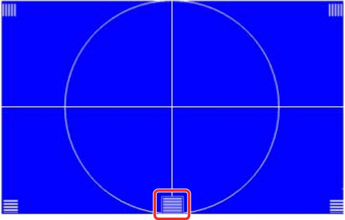
7. Once the center reference point is in focus, check that the corner reference points are also in focus.
