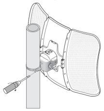
8. Adjust the azimuth and elevation angle of the CPE device to achieve maximum signal strength.
