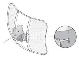
b. Attach the Rear Cover to the reflector assembly. Press upon the Rear Cover at the four positions marked in the diagram below in sequence until it locks into place.
