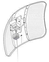
5. Attach the Mounting Bracket to the Rear Cover until the grooves on the Mounting Bracket are positioned over the pins on the Rear Cover.
