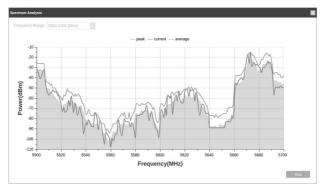
3. When choosing channel/frequency, you should avoid the spectrum with large radio noise. In this example, the recommended channel/ frequency is 112/5560 MHz.
