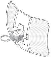
b. Wrap the metal strap around the pole. Use a socket wrench or screwdriver to turn the screw clockwise and securely fasten the strap to the pole.
