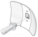
4. Connect the Ethernet cable to the Pharos CPE.
