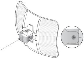
6. Secure the Mounting Bracket to the Rear Cover using M6x79 Hexagon Bolts with Wing Nut and Lock Washer Assemblies.
