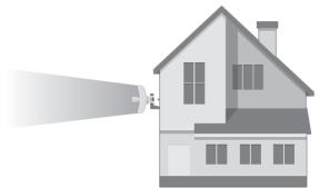
The CPE device without the reflector installed provides outdoor -to-indoor Wi-Fi coverage with the Feed only mode.
