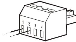
If the contacts are closed, the UPS will turn OFF and power will be removed from the load.
