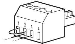
If the contacts are opened, the UPS will turn OFF and power will be removed from the load.
