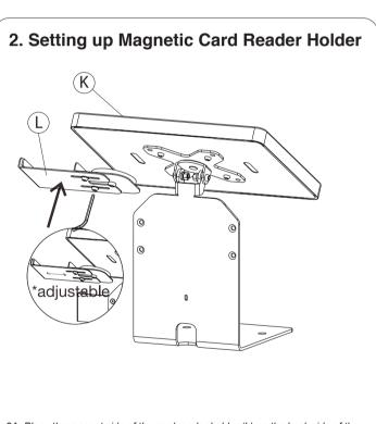
2A. Place the magnet side of the card reader holder (L) on the back side of the enclosure at desired location.
