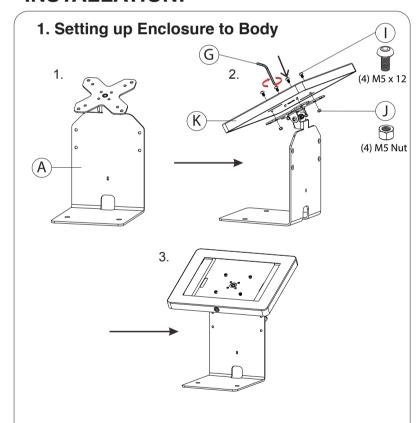
1A. Align kiosk body VESA plate holes to Enclosure VESA holes. Then from above, rotate in screws (I) while holding the hex nuts (J) with your fingers from behind. Rotate
