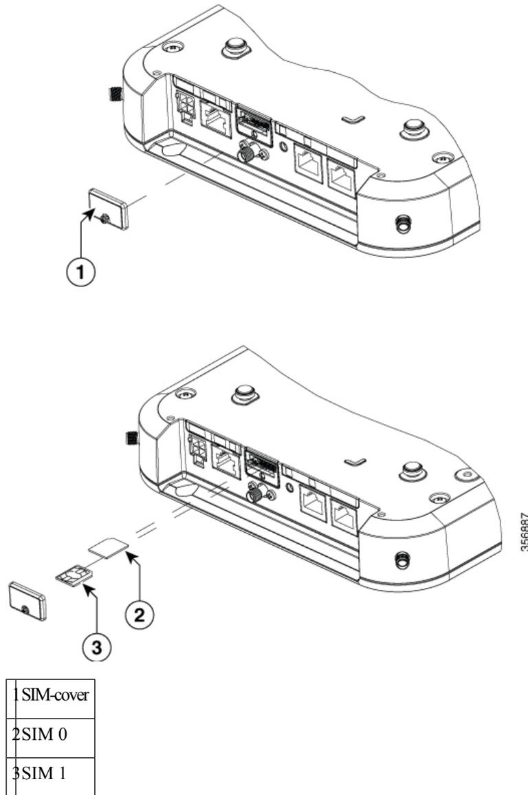
The Cellular Gateway unit supports dual SIM cards behind a panel cover. To install SIM cards, follow these steps:
