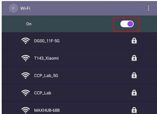
3. Press **▲/▼/◀/▶** on the remote control to select the network's name and connect to the network. The password is needed if it is your first time to use the network. Key in the password and press **Connect**. The device is now connected to the WLAN.
