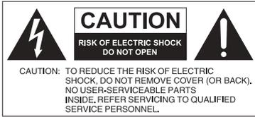
The lightning flash with arrowhead symbol, within an equilateral triangle, is intended to alert the user to the presence of uninsulated “dangerous voltage” within the product’s enclosure that may be of sufficient magnitude to constitute a risk of electric shock to persons.
