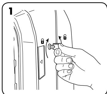
Unlock access panel: to unlock, insert the key provided and rotate counter-clockwise  $\frac{1}{4}$  turn.
