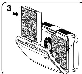
Remove any packaging wrap from the new filter(s) and re-install the filters.
