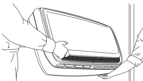
Carefully un-tilt the machine until it is resting vertically, supported by the wall-side bracket, and the removal latch has engaged. The machine may need to be gently slid left or right to ensure the latch is fully engaged. A small click will be heard when the latch engages.
