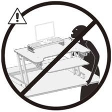
**Warning:** Impact Hazard! Moving Parts can cause serious injury. Raise work surface to top of vertical adjustment before removing equipment. Failure to heed this warning may result in serious personal injury and or property damage.
