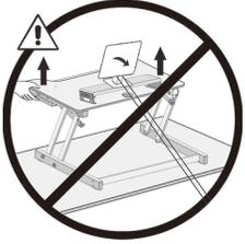
**Caution:** Leave enough slack in cable to allow for full range of vertical motion (15"/38cm). Failure to heed this warning may result in property damage and or personal injury.
