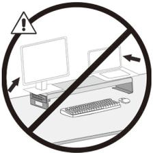
**Caution:** Keep monitor and laptop base fully on the work surface. Allowing any part of base or stand to hang off the edge may result in property damage and or personal injury.
