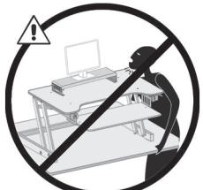
**Warning:** Impact Hazard! Moving Parts can cause serious injury. Raise work surface to top of vertical adjustment before removing equipment. Failure to heed this warning may result in serious personal injury and or property damage.
