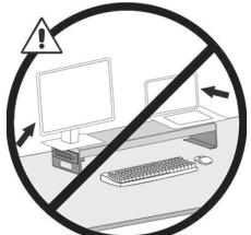
**Caution:** Keep monitor and laptop base fully on the work surface. Allowing any part of base or stand to hang off the edge may result in property damage and or personal injury.
