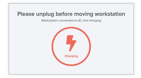
To begin charging your Mosaic, plug the 3-prong power cable into a standard 110-120VAC grounded AC power outlet. The screen will read "Charging" (left) when the machine is successfully charging.
