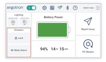
When the Drawers are unlocked, the panel will show Lock and Mute Alarm controls.
