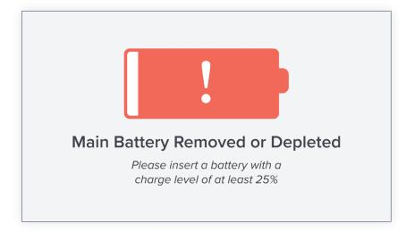
When swapping the battery, the display will read "Main Battery Removed or Depleted" and will beep twice every 5 seconds for 4 minutes prior to entering Standby.
