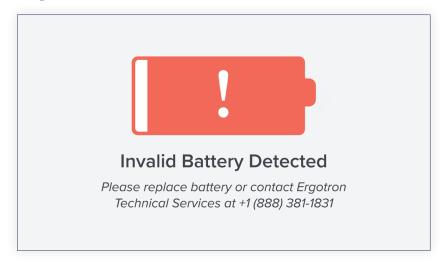
Users will receive the message below on the touch display when the workstation detects an unsupported battery. The workstation will also disable the channel outputs.
