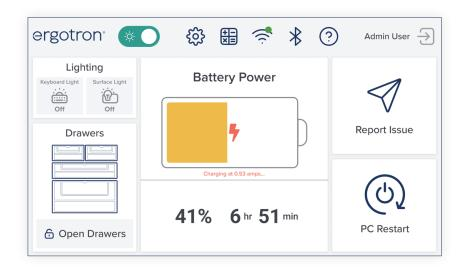
An orange "Charging" will appear below the battery icon on the home screen when a user logs into the workstation, indicating that the battery is charging.
