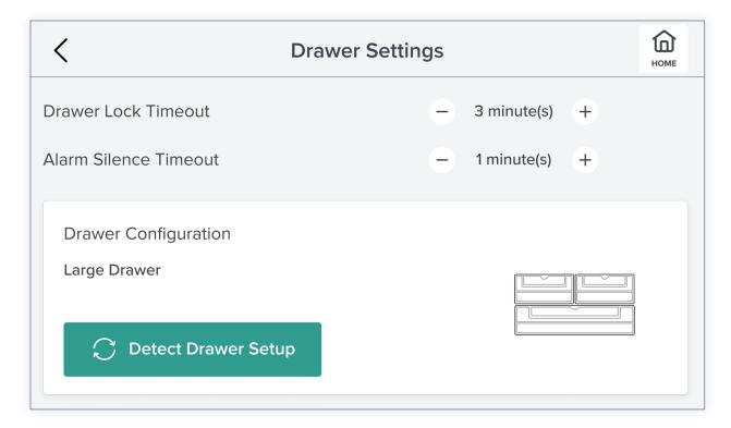
**Drawer Lock Timeout:** This setting determines how long the workstation waits before automatically locking the drawers after they are accessed.
